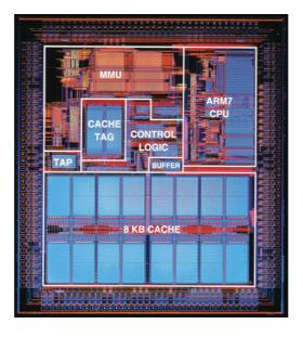
$ARM710 \ \ (25 \text{mm}^2 \text{ en } 0.5 \mu\text{m} \ \ (1995), \, 2.9 \ \text{mm}^2 \text{ en } 0.18 \mu\text{m} \ \ (2000))$
